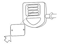
Step 6- Replace the screws (2) fastening the battery cover at the rear of the monitor as shown.
