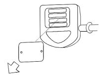
Step 3- Remove Batteries as shown.
